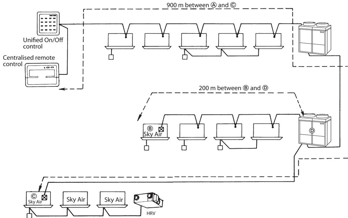
In the above system, the longest wiring extension is 900 m between A and C, which satisfies the limit of 1,000 m. The total length is 1,100 m, that is the total of 900 m between A and C and 200 m between B and C, which also satisfies the limit of 2,000 m. The central controller functions properly, only when both the longest extension and the total length of wiring satisfies the limitation, as shown above.
