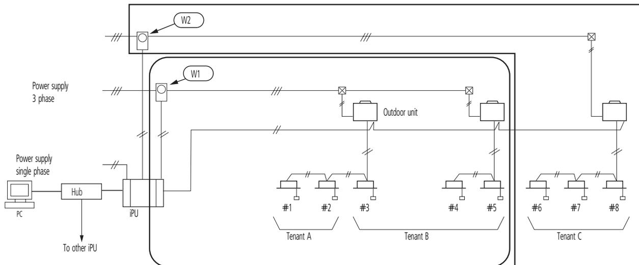
The power input to iPU can be counted with the proportional division system based on the every input of wattmeter. On the above example, watts at W1 and watts at W2 are shared by indoor units #1~#5 and indoor units #6~#8, respectively. (Before the test run goes on, it is necessary to enter the exact power port No. on the address table.)
