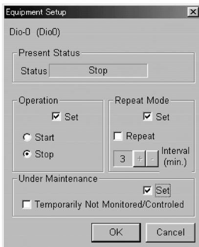
In addition to start/stop operation, supported by all facility equipment, our DIII-NET air conditioners, can be started and stopped with the repeat mode. In this case the outputs start and stop instructions in determined time intervals to make the starting and stopping states of the facility obey the intelligent Manager instructions, regardless of the local operation.
