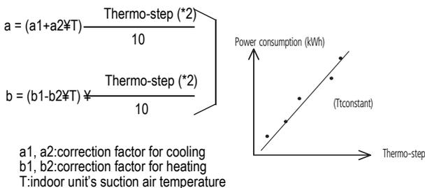
As shown in the left, heat load is calculated from an equation of the first degree which approximates the correlation, among thermo-step, indoor unit's suction air temperature and power consumption, into the linear line under the standard conditions of the unit.
