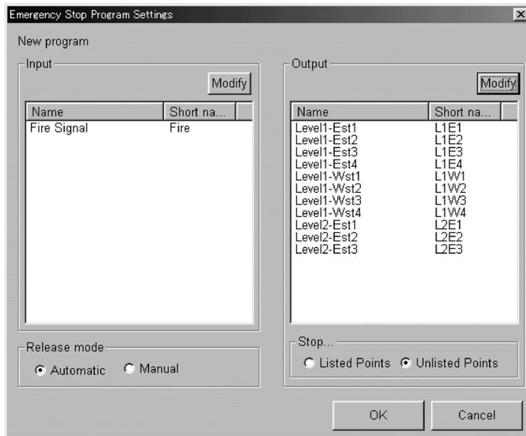
The registration of management items to be targeted for emergency stop can be performed using either method of specifying the management item to stop or of making all management items targets for stopping and then specifying the management item that is out of range.
