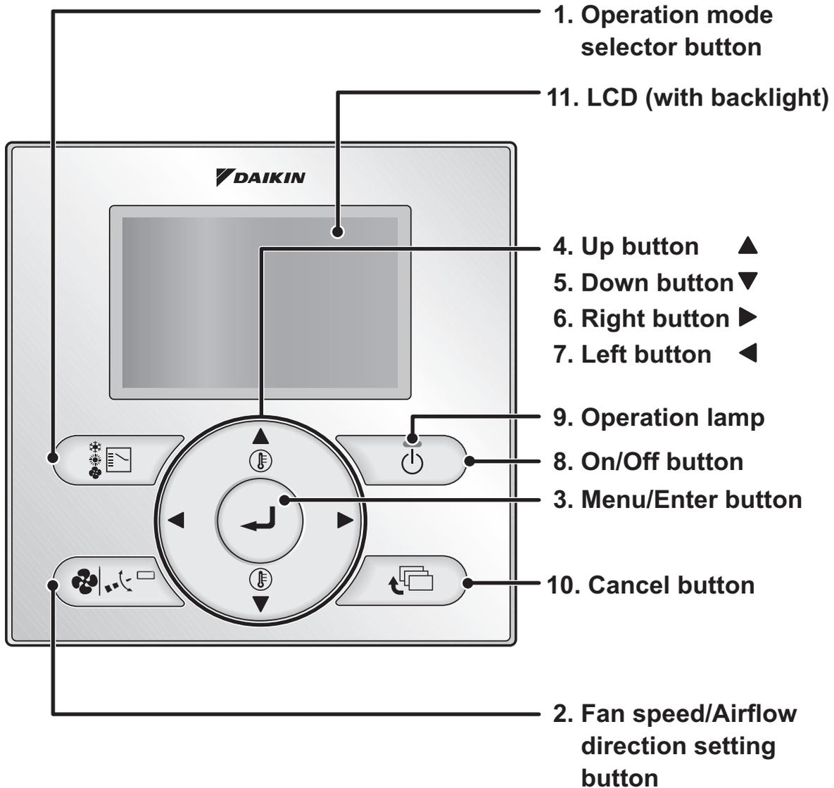
Functions other than basic operation items (i.e., On/Off, Operation mode selector, Fan speed/Airflow direction, and temperature settings) are set from the menu screen.
