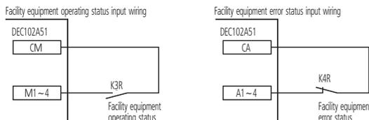
When the switch was set to "Ins." (Instantaneous Output), the operation input terminals M3, M4 and abnormal input terminals A3, A4 are not used.
