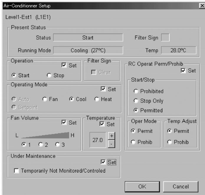
Each of the operations of start/stop, switching of operating mode, changing of temperature settings, switching of enable/disable of individual remote controllers, resetting of the filter sign, clearing of the failure warning and settings for being under maintenance are possible when using our DIII-NET compatible air conditioners.
